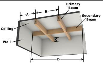
All dimensions are measured to wall faces and to centerlines of beams.
