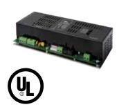
The K1840 & 1841 is a UL Listed, universal input switching power supply capable of delivering a full 192W of continuous power for fire alarm systems. Suitable for charging a range of sealed lead acid batteries from 7Ah to 40Ah, the K1840 & 1841 power supply features complete monitoring of primary and secondary power sources with fully temperature compensated battery charging and battery high impedance monitoring.
